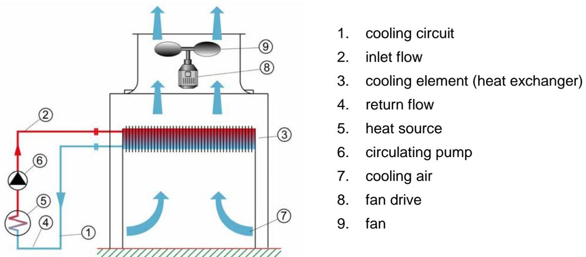
Fig. 1: Sketch of a dry cooler (SWKI, 2005)
